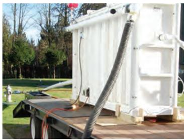
The EPA requires corrosion control at three Company wells. This is currently being addressed by adding sodium hydroxide (NaOH) to raise the water's pH. Using a newer technology we will be adjusting the pH at the new Well 5 using an aeration system. Rather than adding a chemical to the water, this system will remove naturally dissolved carbon dioxide (CO<sub>2</sub>) which raises the pH. Pilot tests verified that the system will also work well at our Wells 3 and 9 which currently use NaOH.
